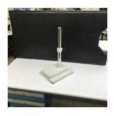
2.) Lower the BOOM ARM (with long side facing up) down onto the base POST.
