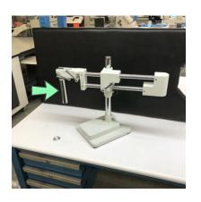
6.) Slide HEAD ASSEMBLY up onto NECK and screw endcap back into place at the end of the NECK.
