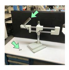
5.) Swing the PIVOT NECK into down position and tightly secure with lever.
