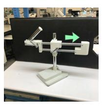
4.) Remove the threaded endcap from the PIVOT NECK and set aside temporarily.
