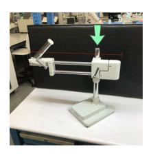
3.) Slide the BOOM ARM out to balance the assembly. Use the lever to secure it's position.
