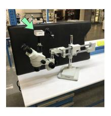
8.) Slide the RING LIGHT up onto the lower part of the HEAD ASSEMBLY and secure it in place using the three thumbscrews.
